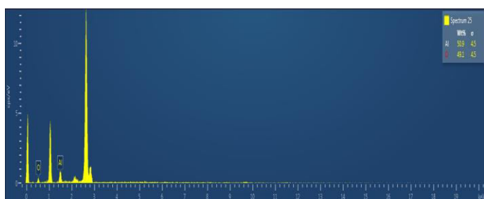
Fig-3.5: EDX image showing the presence of \text{Al}_2\text{O}_3 Nanoparticles
